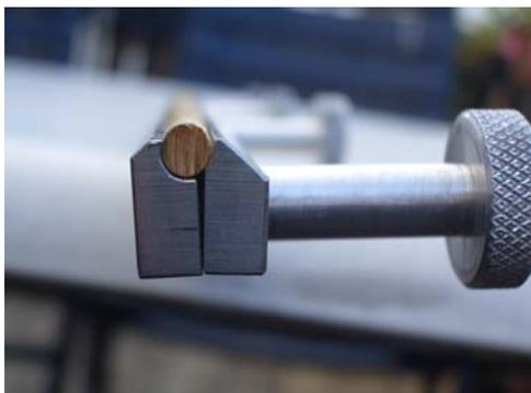
The tool has to be designed according to the size of the section that you want to cut off and the core diameter. This tool gives the best cut. Depending of the size of the section, the type of the wood (hardness) and the precision you want to get, we perform a pre-cut by the following instrument:
