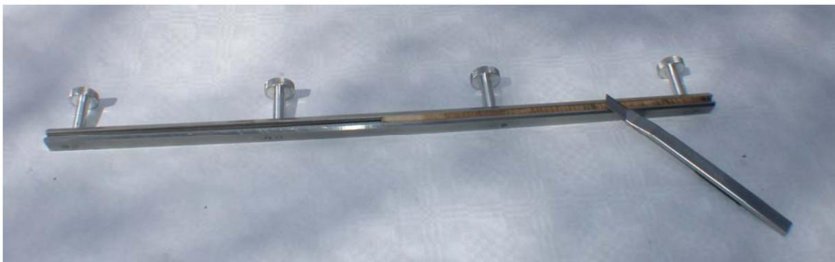
**B) This cutting tool is more advanced. It consists of two formed metal pieces (steel tracks or titan), the core can be fixed very tightly turning the screws.**
