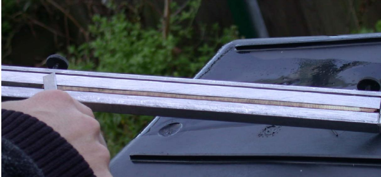
**A) One of our first cutting tool made out of metal. It is a U-shaped bar with a moveable bar inside. One puts the freshly taken core with correct orientation of the vessels in the groove, than the core can be fixed by the metal bar in the middle of the U-shaped bar by turning the screws. Than we use a sharp cutter. This one has been in use since the 80ies. It weighs depending on the metal type between 300 to 600 g.**
